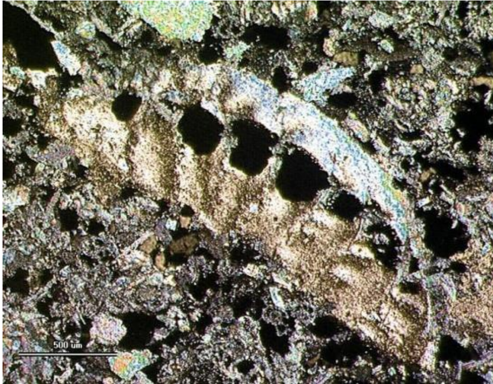
Fig. 7 The structure of limestone. Polarized light, bar. 0.1 mm
