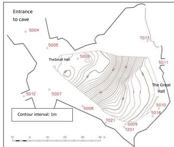
**Fig. 13** Isolines of ground ice in interpolation in R
