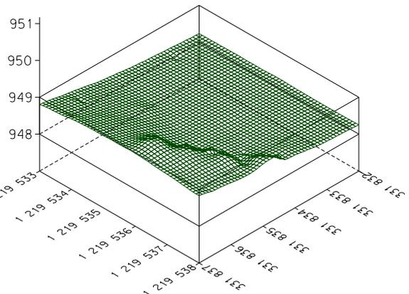
Fig. 6 The spatial model of ice surface obtained from the 3D scanner
