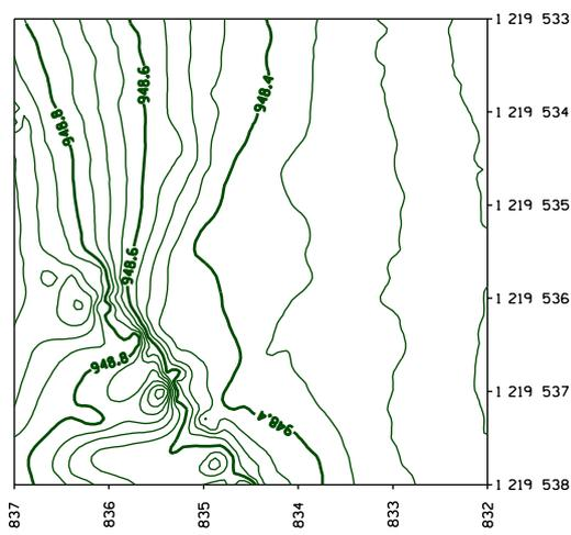
Fig. 8 The ice surface level lines obtained from the terrestrial laser scanning
