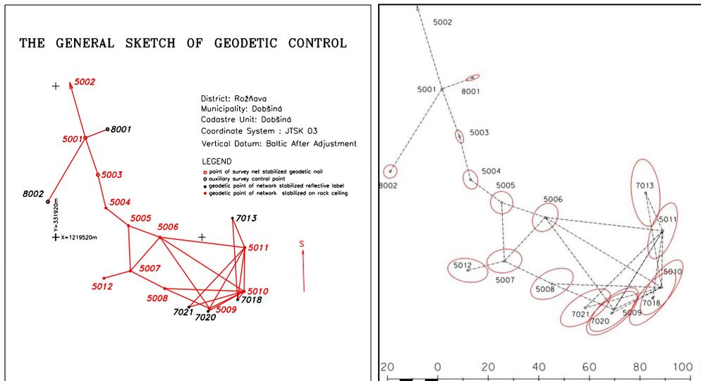
Fig. 4 The general sketch of geodetic control, Standard errors ellipses
