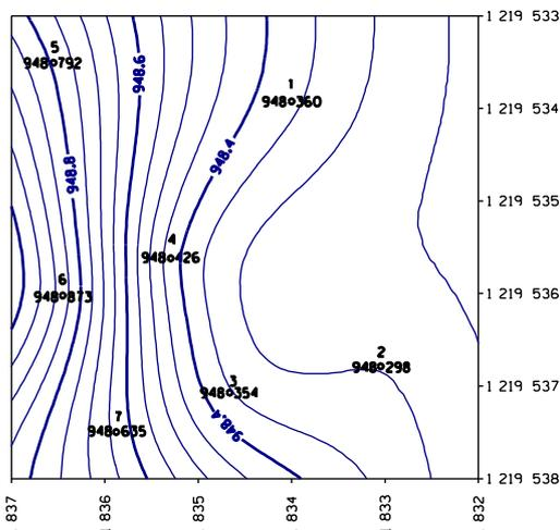
Fig. 7 The ice surface level lines obtained from the tacheometry
