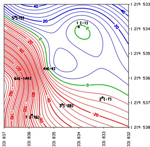
Fig. 9 The correction isolines for the points assigned by terrestrial laser scanner
