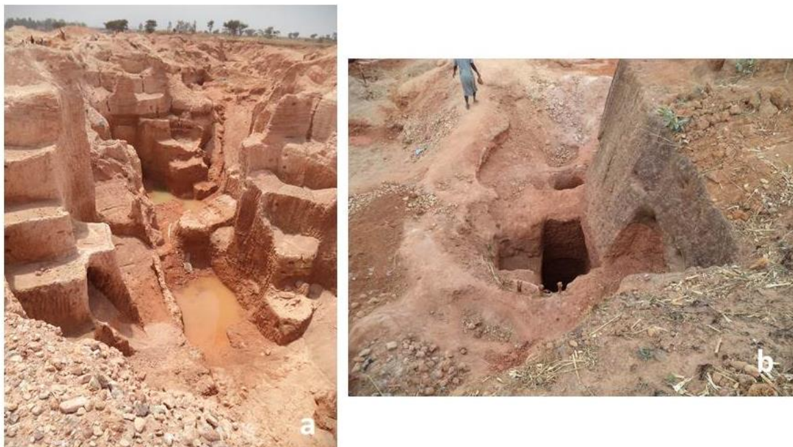
Fig. 5 Benching in an open pit mining for tin in Bassa during the colonial mining era of the pre-1960s
